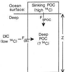
Model of deep-ocean POC formation from dissolved inorganic carbon (DIC) and sinking POC sources. Within the deep ocean, sinking and suspended POC are not differentiated.  $F_{\text{spec1}}$ , areal flux rate of sinking POC through the surface/deep ocean boundary;  $F_{\rm dic}$ , areal flux rate (uptake) of deep DIC into POC.
